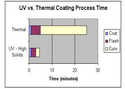
Figure 1: Comparison of general processing times for UV and thermal cure coatings
